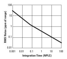
Auto-zero on for NPLC ≥ 1. See manual for additional noise characteristics.
